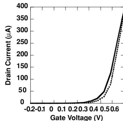
Fig. 2  $I_d$ - $V_g$  curves for elastic scattering processes (solid) and a combination of elastic and inelastic scattering (dotted) included for deeply buried dopants
