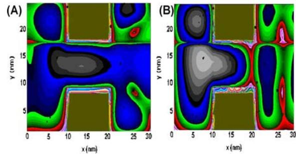
**Fig. 4** Electron density in the  $xy$ -plane taken at a depth of approximately 5 nm into the InAs device layer for (a) elastic and (b) combined processes
