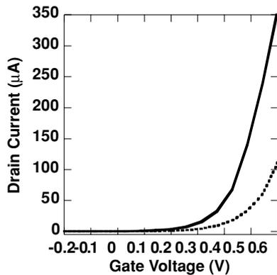
**Fig. 3**  $I_d$ - $V_g$  curves for elastic scattering processes (solid) and a combination of elastic and inelastic scattering processes (dotted) included for dopants near the source-channel interface
