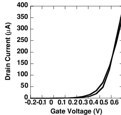
Fig. 1  $I_d$ - $V_g$  curves with only elastic scattering processes included
